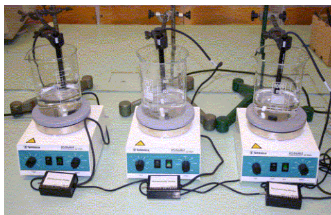
Figure 2: Experimental design for diffusion experiment with three parallel samples and three sensors.
